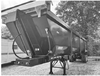
'26 Kruz Terminator, 38'x96"x66", Hardox 450, steel, 2-way gate, Center Point spg. susp.
